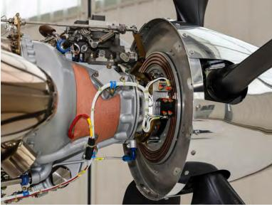
THE NEW, digitally controlled propeller governor-dubbed "R2-D2" by some—sits atop the prop gearbox (above left), fed only by a wiring harness. Earlier PC-12s make generous use of pushrods and other mechanical controls (above right) to adjust power, fuel flow, and propeller rpm. A Hartzell (right) helps give the more efficient, 1,200-shp Pratt & Whit-
