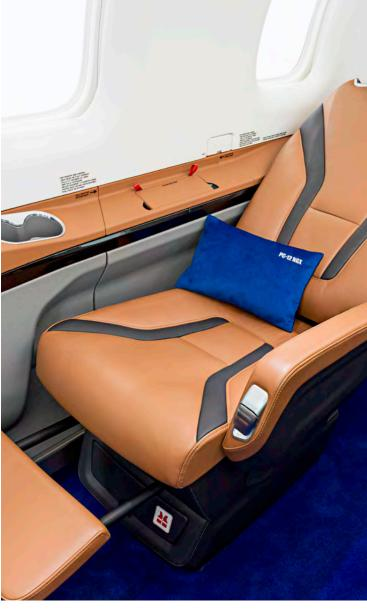
THE NEW PC-12 NGX retains Pilatus' signature large aft cabin door (above) but there are many new enhancements as well—like the redesigned leather seats (above right) with optional footrests, new sidewall ledges with oxygen mask stowage compartments, downwash lighting, and cabin windows 10 percent larger than previous models. All cabin seats are fitted with quick-release hardware, where before only the last two seats had this feature.
